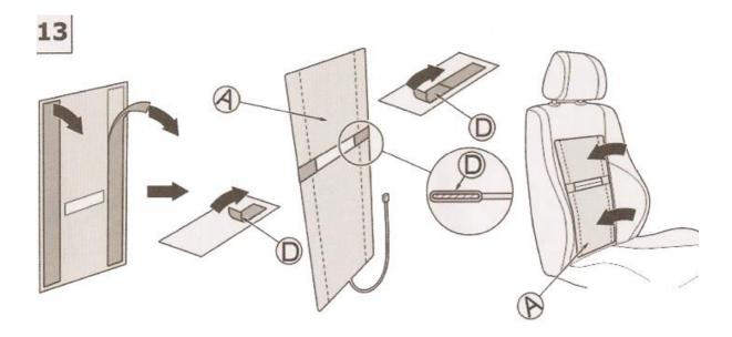
The electrodes on the ends of rectangle aperture (s) must be enwrapped with doubt-coated adhesive protection tape  $\mathbb{O}$ .
