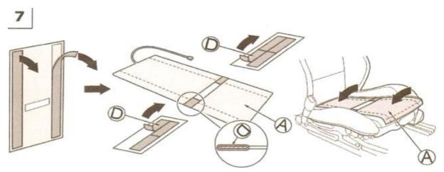
The electrodes on the ends of rectangle aperture (s) must be enwrapped with doubt-coated adhesive protection tape  $\mathbb{Q}$ .
