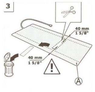
If there are fillisters for trimming wires on the seat or backrest, the heating area of pad within the two electrode tapes should be delineated with pencil or marker pen and cut into a rectangle aperture with 40mm width as illustrated in 3.
