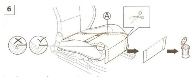
Superfluous parts of the pad must be cut off.
