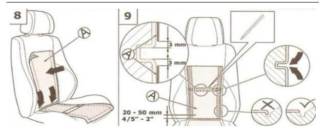
The backrest of heating pad should be unfold as illustrated in 8
