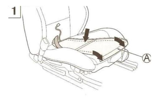
The heating pad should be unfold as illustrated in above
