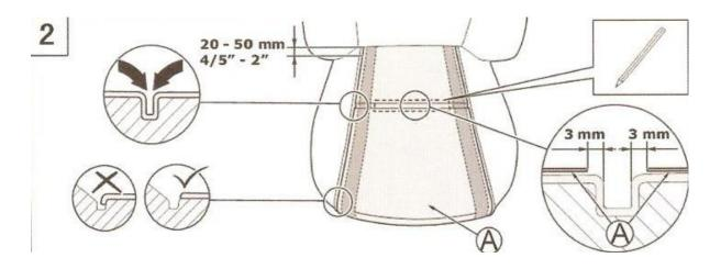
There are at least 3mm between the pad and fillisters after the pad is unfolded nicely. The heating area can not be put inside of any fillisters.
