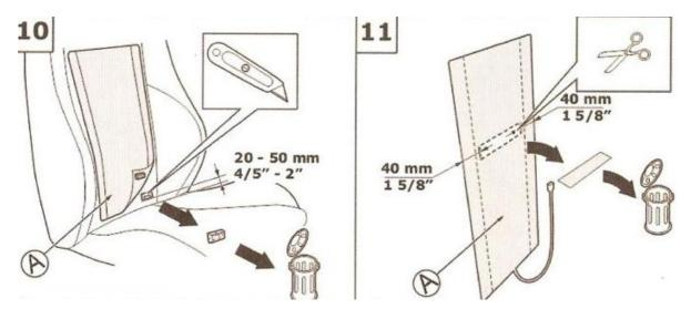
The foam opposite to the temperature controller should be cut into a hole, in order to level the pad.
