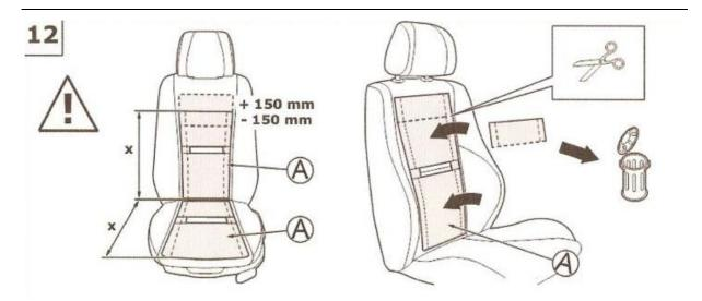
There are ±150mm cutting deviations of either seat or backrest. Superfluous parts of the pad must be cut off. The backing should be ripped when the pads are installed.
