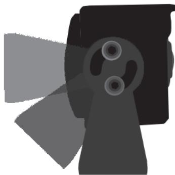
Fasten the camera in a suitable location as surface-mounted camera. The bracket can be adjusted in several positions with 4 small screws.
