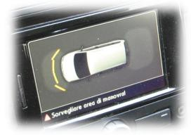
The system interacts with the car, automatically showing the display front and rear, depending on the type of installation performed (rear, front or rear and front only).
